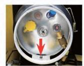
The locator pin in the locator hole restricts the movement of the cylinder. This decreases the wear and tear on the hose and connection fittings.
