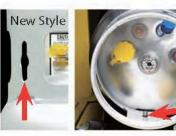
Place the bracket locator pin in the cylinder locator hole.
