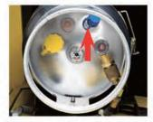
When the cylinder is positioned correctly, should the relief valve open, the propane would expel away from the driver.
